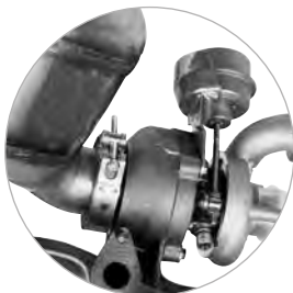
Automotive: Turbocharger – catalytic converter connection
